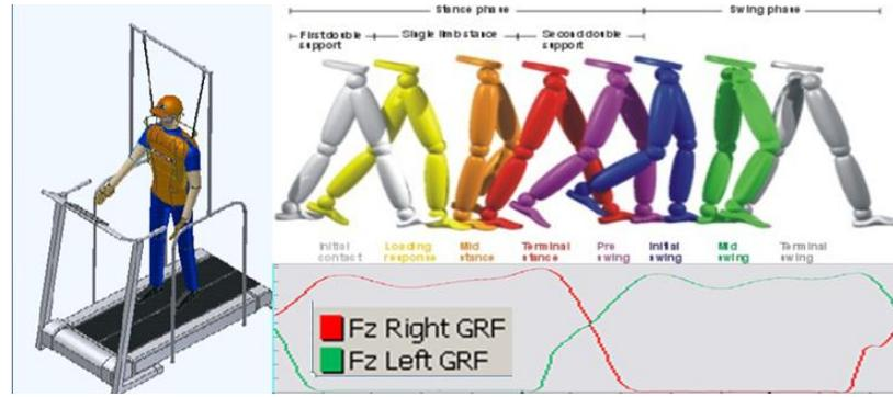
Figure 1 Instrumented Treadmill, Human Gait phases and a typical vGRF Chart
