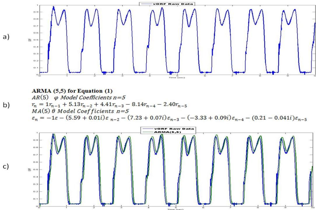
Figure 3 Subject 1: a) Show Signal vGRF Raw Data as Data-Driven b) ARMA (5, 5) Equation calculate for Model Driven, c) Both charts compared for the Data-Model Driven (The first from left to right is raw data and the second the ARMA)
