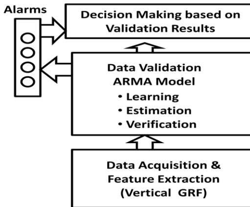
Figure 2 Steps for Sensor Validation using Model and data driven methods
