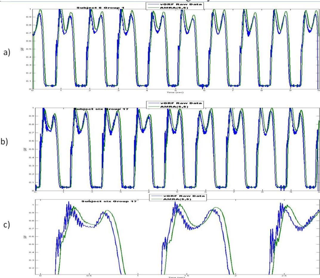
Figure 5 On subject 6 a) Group 1 is acceptable, b) Group 17 a bigger noise is detected and a warning signal emitted. c) Group 17 with a zoom where the excess of noise was detected.
